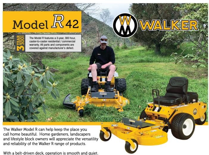
Featuring a powerful 22 HP Kohler KT722 with SmartChokeTM technology, this machine is a premium Walker Mower. Tilt-open seat and tilt-up deck are designed for easy maintenance access.
